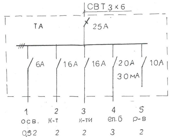
P инст 9.5 kW P<sub>p</sub> = 6 kW
